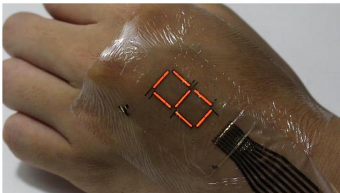
*E-skin at work. Sensor readout shown on PLED display attached to the hand.*
