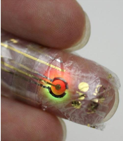
*Light from red & green PLEDs is directed into the finger. Photodetectors catch the reflected light from inside the finger and provide a measure of blood oxygen. The output of a detector is shown in the photo below.*
